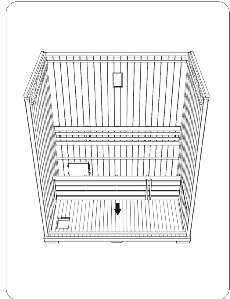
FIG 7 – Installing front bench panel
